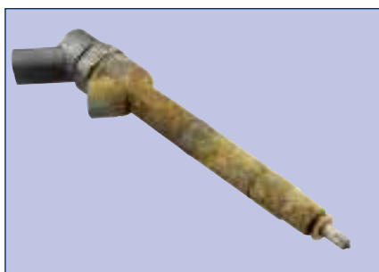
Injector: Starke Korrosion
